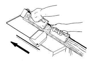
Use hold down/push blocks for wood under 3 in. wide. Position them so you have control of the work piece at all times and so they do not contact the guard or the cutter head.
